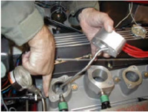
Figure 4 - Injector body
