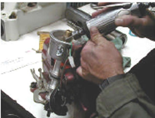
Figure 14 – Grinding out 7 of the 8 vanes.
