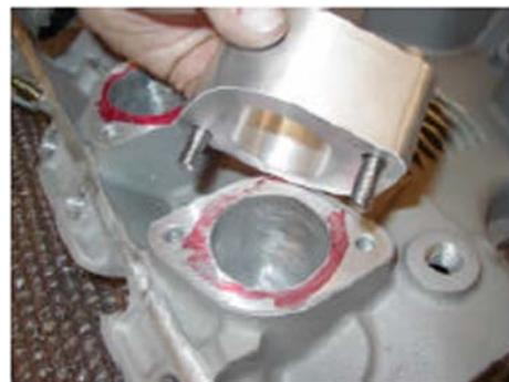
Figure 6– Match porting injector with intake manifold
